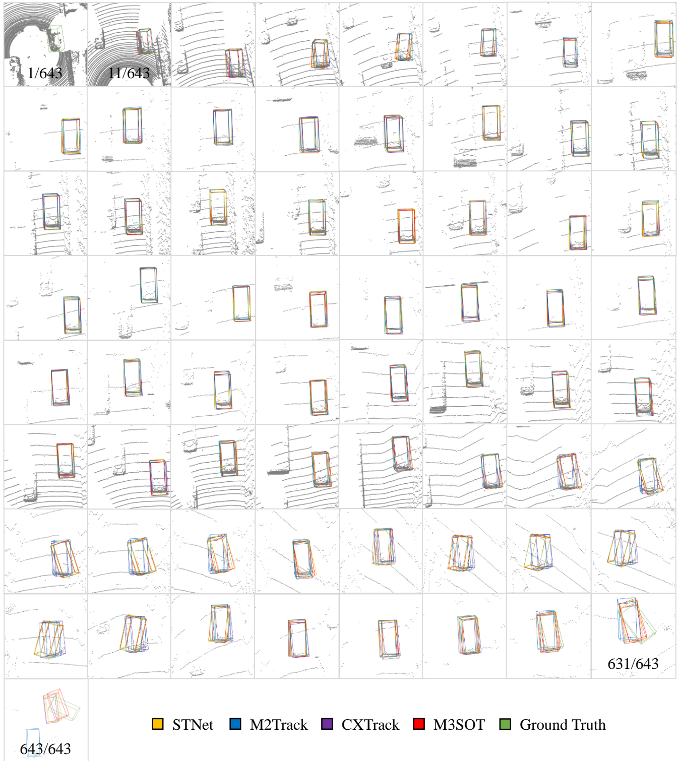
Figure 10: Visualization of long-range tracking results from different methods on KITTI. A scene is switched every 10 frames.
