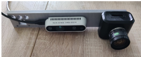
Fig. 4: Sensor setup of the ATIS and Intel Realsense, enabling the development of a synchronized bimodal dataset for gesture.
